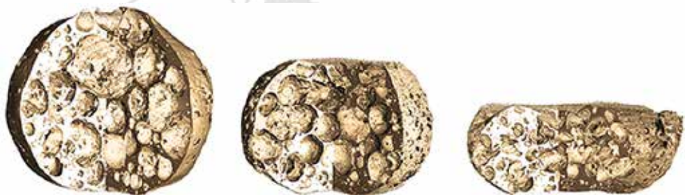
Visualisation of a deformed APM sphere - reconstructed 3D image captured at 0 %, 25 %, and 50 % of overall compressive strain.
