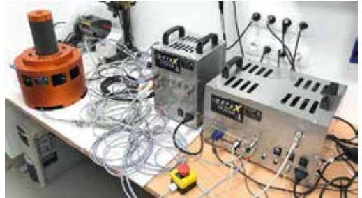
DETEX testing solution: the control unit with the servo motor expansion module for control of the uni-axial loading device (nominal force 25 kN) suitable for X-ray imaging.
