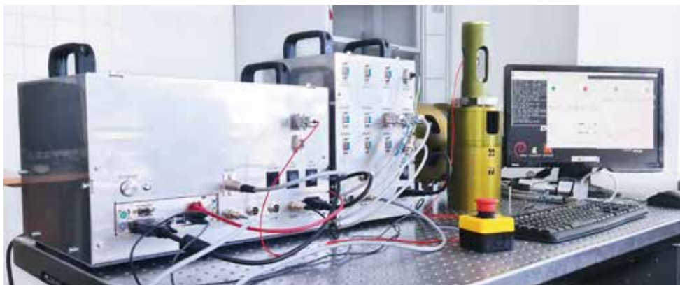
Control unit (mini-ITX configuration) with the stepper motor expansion module for control of the uni-axial loading device (nominal force 3 kN) suitable for X-ray imaging.
