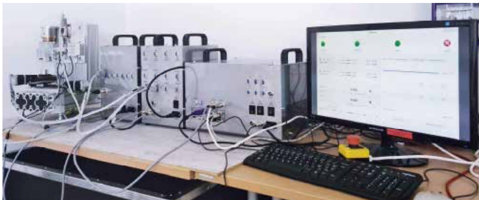
Control unit (micro-ATX configuration) with the servo (voice-coil actuator) motor and stepper motor (two-axis table) expansion modules for the control of the micro-indentation stage.
