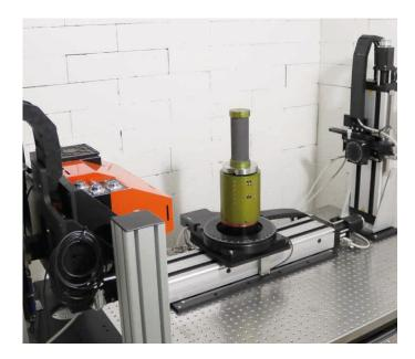
The device can be fully integrated into customized as well as standard imaging systems. Control is performed by the RaPo software supporting monotonic, low-cycle, and creep testing.
