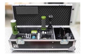
The device is delivered in wheeled safety transport case. Loading frame can be customized and equipped with various accessories.
