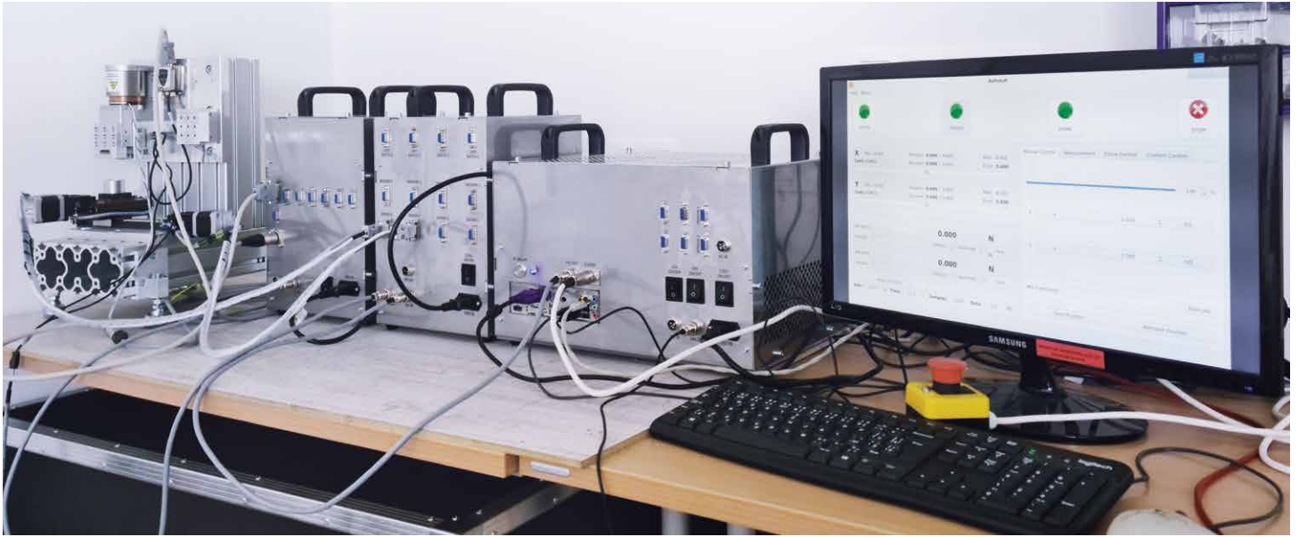
Control unit (micro-ATX configuration) with the servo (voice-coil actuator) motor and stepper motor (two-axis table) expansion modules for the control of the micro-indentation stage.
