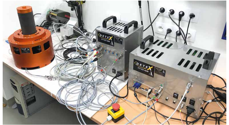
DETEX testing solution: the control unit with the servo motor expansion module for control of the uni-axial loading device (nominal force 25 kN) suitable for X-ray imaging.
