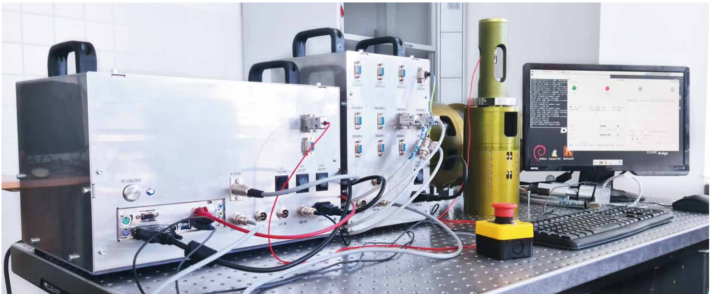
Control unit (mini-ITX configuration) with the stepper motor expansion module for control of the uni-axial loading device (nominal force 3 kN) suitable for X-ray imaging.
